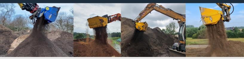
The HDX range. All models in this range are 1500mm wide and have additional hardox wear plates. The models have a unique design allowing for loader conversion. Using a Kustom Konnect interface the buckets can have a dual interface system.
