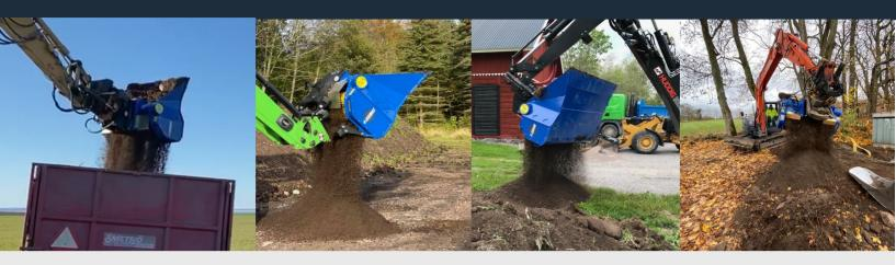
The MAX range, known for the longer wider cutting edge. These screening buckets are the largest capacity buckets available. The specialist design makes it easier to pick up longer smaller piles of material. Perfect for padding and backfilling, the MAX buckets can screen directly into the trench.
