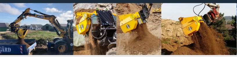
The HE range, designed for heavier excavators but, has the option for loader conversion. These buckets have increased size and capacity in comparison to the E range due to an increase in rotor quantity and length.
